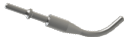
AIR HAMMER PUNCH - Long radius, 3/8" chuck. For removal of conical tools from blocks. Hardened tip provides long life. Fits air-hammer guns with 3/8-inch chucks.
