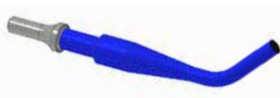
AIR HAMMER PUNCH - 1/2" chuck with hardened tip. For removal of conical tools from blocks. Fits light-duty and heavy-duty air-hammer guns with 1/2" chuck.
